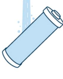
Rinse the filter under running water for 10 seconds (make sure it's soaked).
