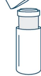
Remove filter from the filter pod and dispose of the outer packaging.
